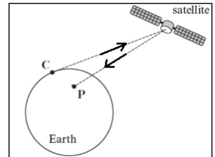
To send a signal from C to P, the signal must travel from C to the satellite and relayed back to P. To send a signal a greater distance then more than 1 satellite can be used.
