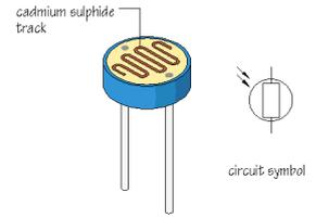
If the LDR is connected as part of a circuit as shown in the diagram then as the light level is increased its resistance falls and the proportion of the input voltage across it will also fall.
