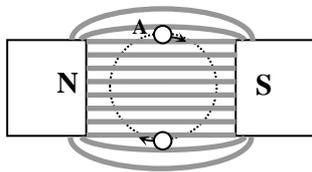
The coil is **not** cutting any field lines – its just moving along with them in the North-South direction. This means that **NO** voltage is produced.
