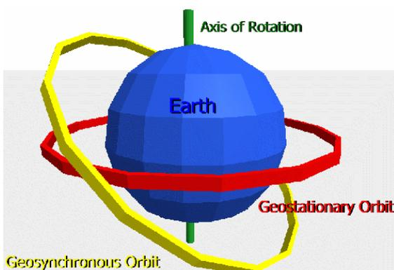
The distinction being that while an object in geosynchronous orbit returns to the same point in the sky at the same time each day, an object in geostationary orbit never leaves that position. A base station can be in constant communication with a geostationary satellite but only once every 24 h with a geosynchronous satellite.
