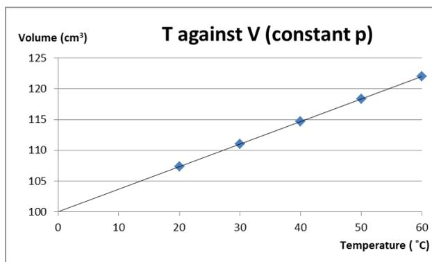
If the temperature is measured in **KELVIN** rather than degrees Celsius (see later on !), the graph would show that the volume doubles when the temperature doubles. This means that volume is directly proportional to the temperature, and hence we can write :
