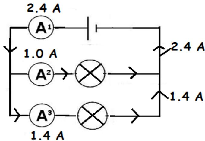
The value of the current in the two branches adds up to the total current flowing, i.e. ( $A_1 = A_2 + A_3$ ) or ( $2.4 = 1.0 + 1.4$ ).
