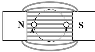
The coil is cutting through magnetic field lines at its greatest rate, and so this is when the maximum voltage/current is produced.
