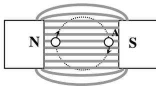
Once again lines are being cut at maximum rate, but side "A" of the coil is now cutting **down** through the magnetic field. This changes the direction of the voltage.
