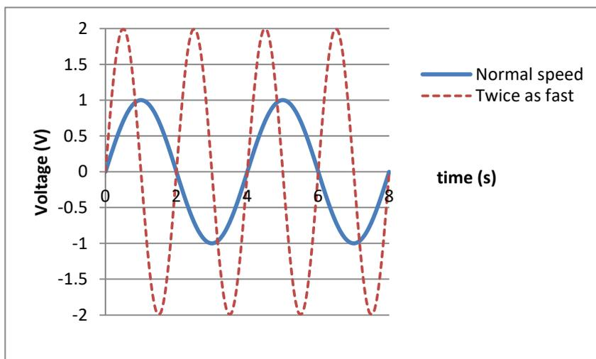
Notice the effect of **doubling** the speed of rotation of the generator.
