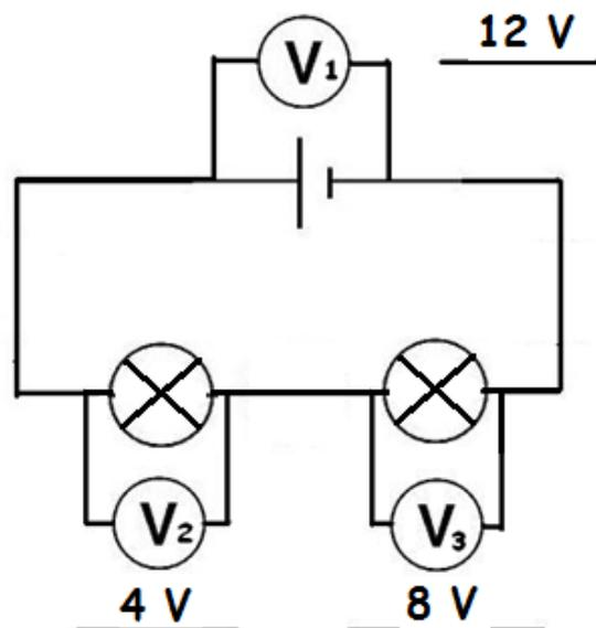
The voltage across both components/bulbs here adds up to the voltage across the supply/battery i.e. ( $V_1 = V_2 + V_3$ ) or ( $12 = 4 + 8$ ).
