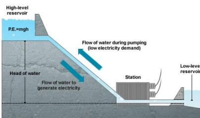
A fast-response hydroelectric power station (pump-storage). Electricity can be imported from other European countries in times of high demand.
