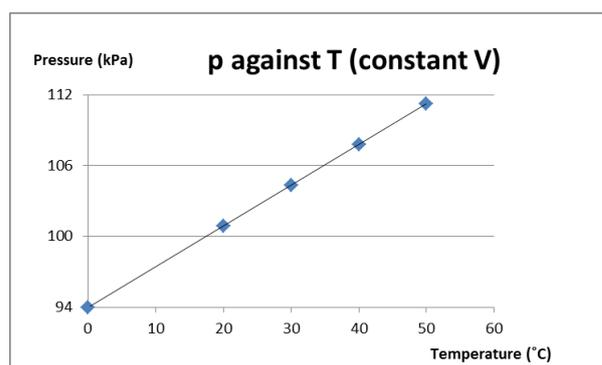
If the temperature is measured in **KELVIN** rather than degrees Celsius (see later on !), the graph would show that the pressure doubles when the temperature doubles. This means that pressure is directly proportional to the temperature, and hence we can write :
