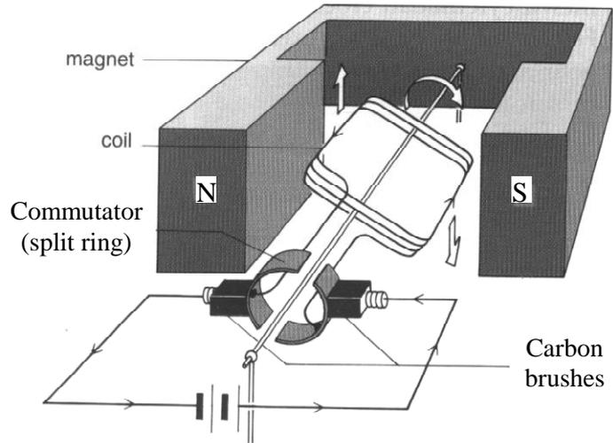
The split ring commutator reverse the current every half turn and ensures that the force on any wire on the left hand side of the motor is always directed upwards, and that the force on the right hand side is always downwards. This makes sure that the coil turns continuously in one direction.
