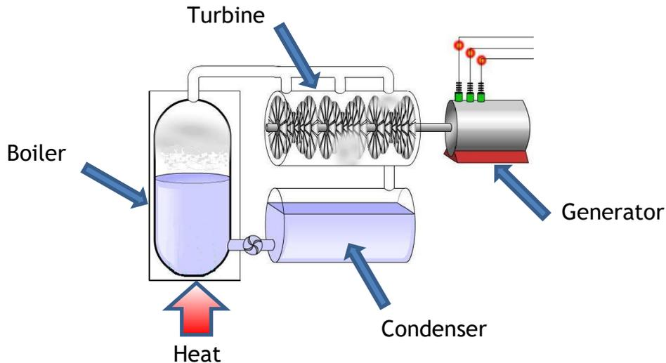
Coal, oil & gas power stations work like this by burning the fuel.
