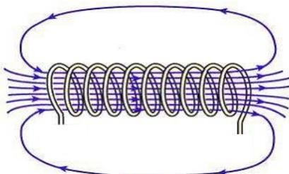
Notice that the field lines **inside** the coil are almost straight and parallel – this shows the magnetic field has a constant strength in this region.
