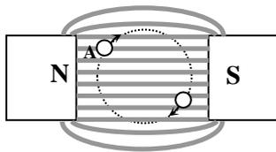
Side "A" of the coil is still cutting **upwards** through magnetic field lines, and so the voltage is still positive. However, because of the angle, the coil isn't cutting the lines as quickly as before, and so there's less voltage.
