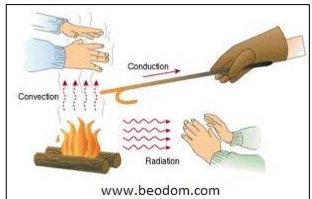
**Conduction:** In conduction the thermal energy flows through the object itself. It takes place in solids and liquids.
