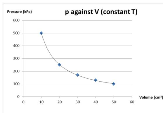
As the volume decreases, the pressure increases. In fact, you can see from the graph that if the volume halves, the pressure doubles. This means that pressure is inversely proportional to the volume, and hence we can write :
