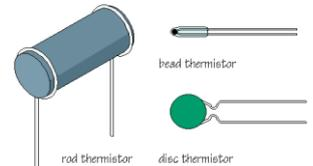
The resistance of most common types of thermistors **decreases** as the temperature **increases** :
