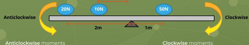
$20N \times 2m = 40Nm$ 10N x 1m = 10Nm
