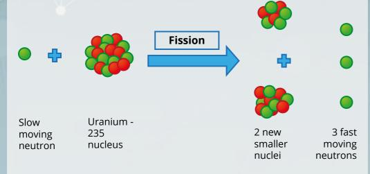
In a fission reaction **one neutron** starts the reaction and **2 or 3 more are released**. In a nuclear reactor these neutrons can go on to **cause another reaction**. If this proses in not controlled this **chain reaction** can become out of control and cause a meltdown.
