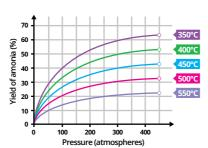
The graph shows that a lower temperature and higher pressure would produce the best theoretical yield
