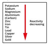
Gold and silver are examples of metals that are found native. The most reactive metals are extracted by electrolysis, while those towards the middle of the reactivity series can be chemically reduced.
