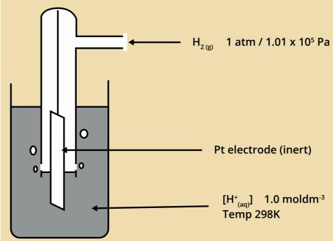
By convention the electrode process at the platinum electrode is taken as the standard and other potentials are measured with respect to it.
