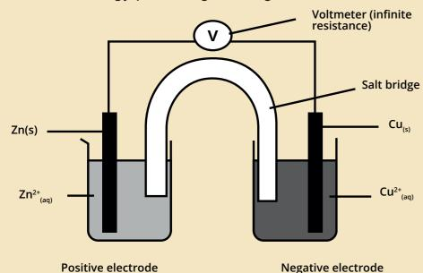
The salt bridge allows ions to flow from one solution to the other while the two solutions are kept separate. The salt bridge is filter paper that is soaked in potassium nitrate solution. All potassium salts and all nitrates are soluble so no precipitate can form in the salt bridge stopping the flow of ions.
