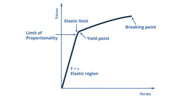
In metals it is important to understand edge dislocations and ductile fractures. Edge dislocations are where there is an extra plane in the crystals, plastic deformation occurs when the **dislocations move** due to the large stress. Ductile fractures (necking) is where the number of edge dislocations increases and causes the elongation of the metal which increases the stress at the neck (smaller A).
