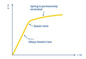
The relationship F = kx can be used to calculate the extension up to the elastic limit. k is the spring constant and represents the stiffness of the spring.
