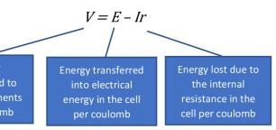
The total current in the circuit can be calculated using this
