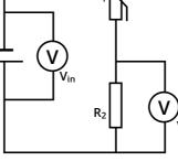
Where V is the **output voltage across the resistor R**, in the example above R<sub>2</sub>.
