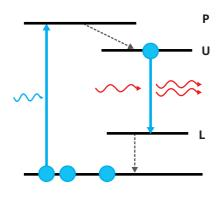
Population inversion is easier to create in a 4-level system as stimulated emission occurs between level 3 and 2 and level 2 is almost always empty. Therefore, only a small number of electrons need to be pumped to a high level to ensure population inversion.
