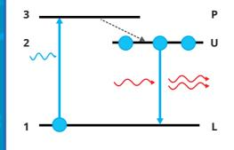
Electrons are pumped to level 3, which is not stable, so the electrons quickly drop to level 2.
