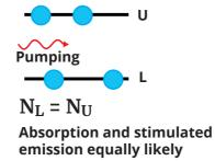
In a 2-level energy system, it is not possible to create a **population inversion** because the best it can create is  $N_L = N_u$ . After this has been reached, the pumping photon is equally likely to cause absorption or stimulated emission.
