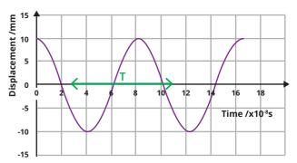
This graph shows how the **displacement of a specific point** varies with time. This example is for the point labelled P on the wave as above.
