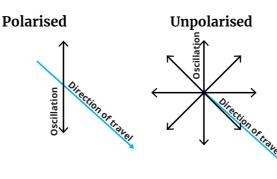
polaroid the intensity that passes through the second would vary between maximum, when the polaroids are parallel, and 0, when the polaroids are perpendicular.
