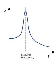
Resonance can be **useful**, for example, microwaves with a frequency similar to the natural frequency of water molecule vibration are used in microwave ovens to heat the water molecules.
