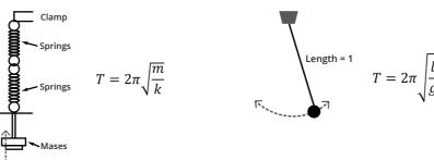
You must be able to describe using the apparatus to calculate *k* or g, as well as using the equations.
