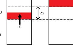
where *p* is the constant pressure in the system and  $\Delta V$  is the change in volume of the gas.
