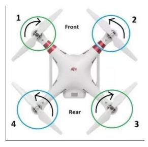
To stay level the total upward force must not change.
